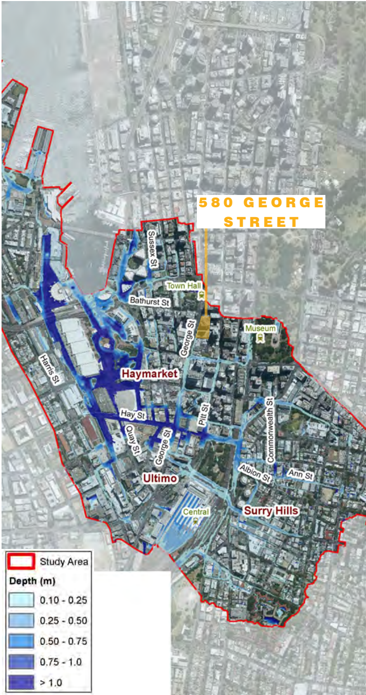
PEAK FLOOD DEPTH PMF DESIGN FLOOD EVENT
